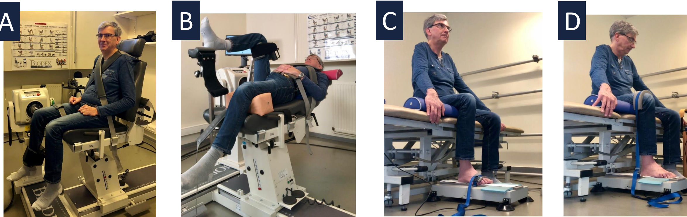
Evaluation of knee and hip flexors and extensors using an isokinetic dynamometer (Biodex System 4 Pro, Biodex Medical Systems, Shirley, NY, USA) (A–B), and ankle dorsiflexors and plantar flexors using a dedicated ankle dynamometer (MyoAnkle) (C–D). Photos displayed with patient consent.
